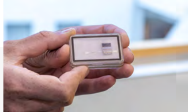
Microelectrode array in package with printed circuit board and connector for electrical connection
